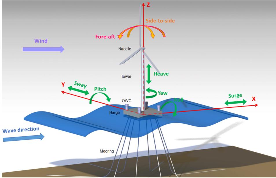
Fig. 1: Barge-type FWT-OWCs configuration.
