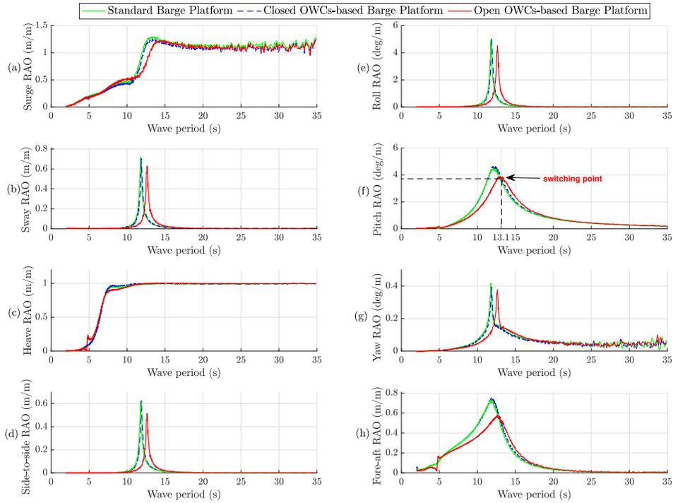
Fig. 3: RAOs at the wind speed of 18 m/s and the wave direction of zero deg. for the following motions: a) Surge. b) Sway. c) Heave. d) side to side movement. e) Roll. f) Pitch. g) Yaw. h) Fore-aft.
