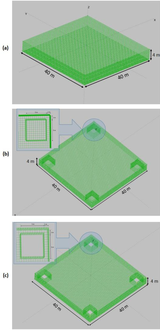
Fig. 2: Substructures configuration (a) Standard barge substructure. (b) closed OWCs-based barge substructure. (c) open OWCs-based barge substructure.
