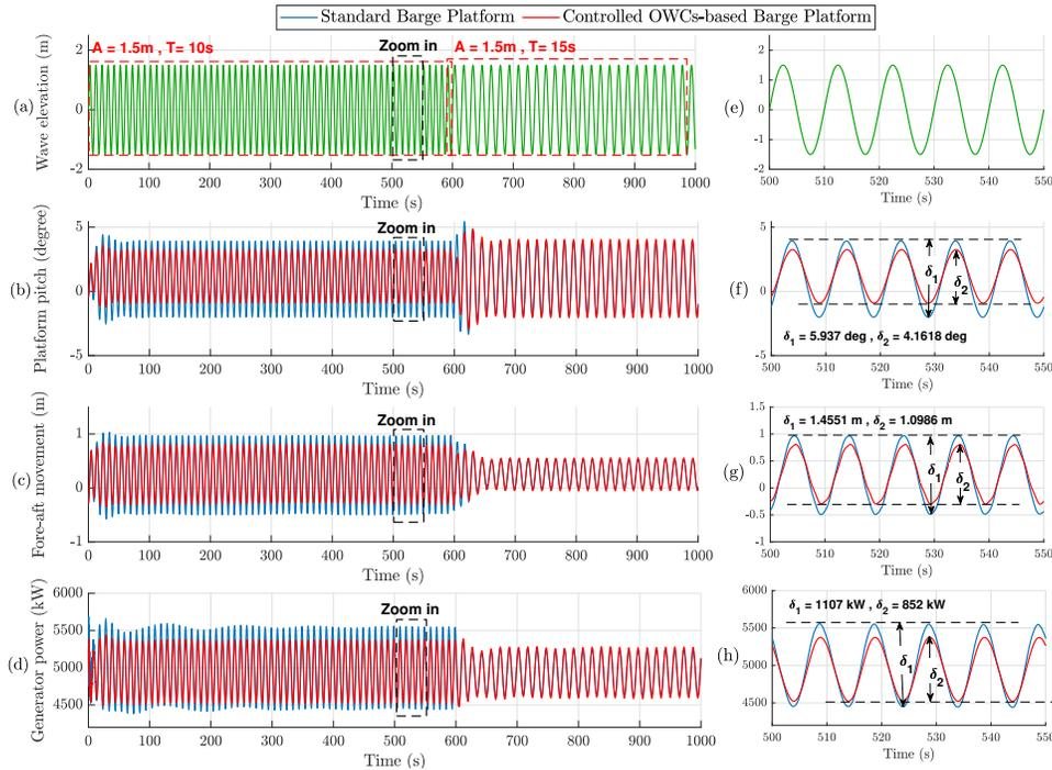
Fig. 4: Condition observed at above-rated wind speed of 18 m/s: a) Wave amplitude. b) Substructure's pitch. c) Fore-aft movement. d) Generator's power.
