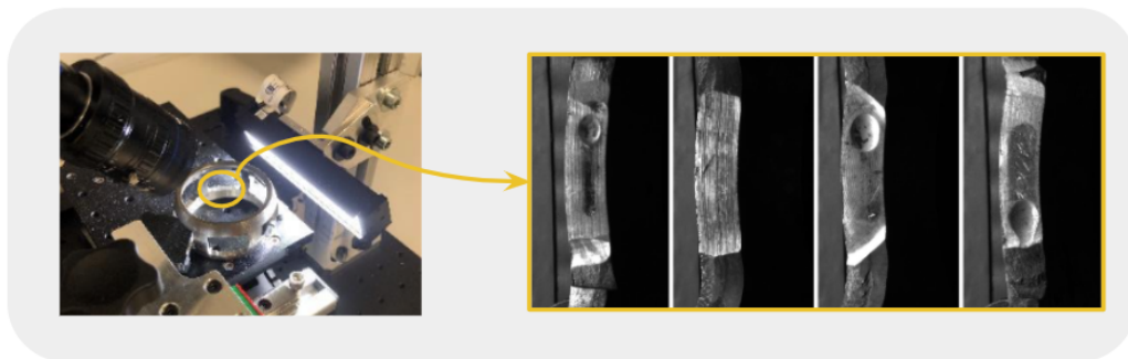
Figure 4.2: CARJAULAS acquisition system and an example of the wear images obtained.
