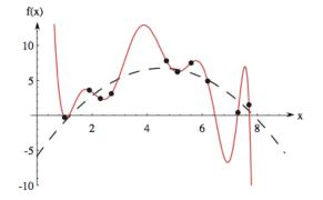
Figure 3.4: The "training data" (black dots) were selected from a quadradic function plus Gaussian noise, i.e.,  $f(x) = ax^2 + bx + c + \epsilon$  where  $p(\epsilon) \sim N(0, \sigma^2)$ . The 10th degree polynomial shown fits the data perfectly, but we desire instead the second-order function f(x), since it would lead to better predictions for new samples.
