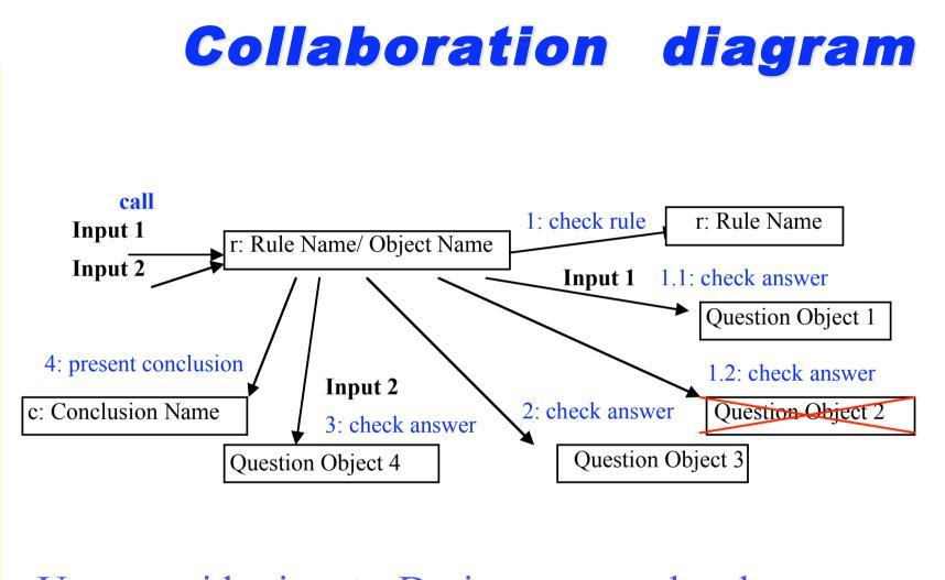
User provides inputs. Design users and end users can observe input effects on rules and conclusions.
