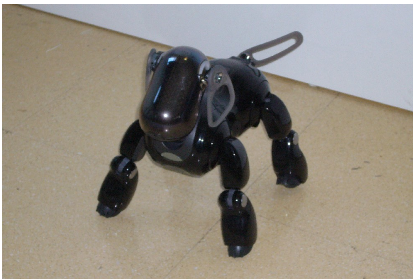
Figure 3.13: Initial configuration of the joints of the Aibo
