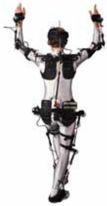
Figure 2.5: Example of electromechanical suite from Gypsy
