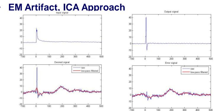
Input signal (ICA extracted EM artifact); Desired signal (channel response); Output signal (EM artifact at desired channel) and error signal
