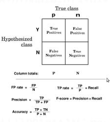
Figure: A confusion matrix and several common performance metrics that can calculated from it.
