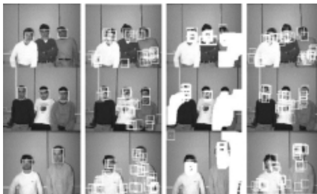
Figure 4-7: Face localization in some of the test images from our database (from left to right): ground truth face pixels, using the fingerprints of the mean face pattern, using PCA and using the combination of all pattern fingerprints, respectively
