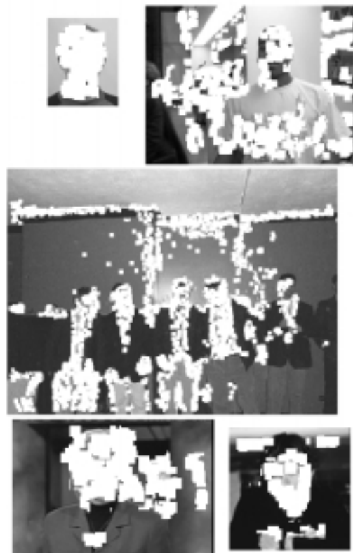
Figure 5-5: Results of the face localization with the HMM approach on the CMU images, using the face patterns displayed in fig. 5.1.
