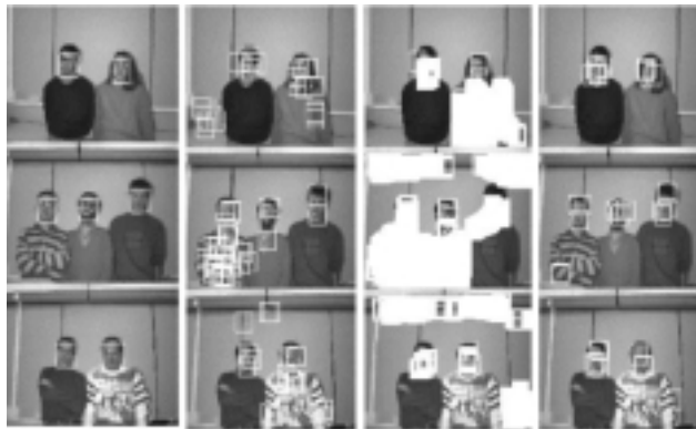
Figure 4-6: Face localization in some of the training images from our database, from which the face patterns have been extracted (from left to right): ground truth face pixels, using the fingerprints of the mean face pattern, using PCA and using a combination of all pattern fingerprints, respectively.
