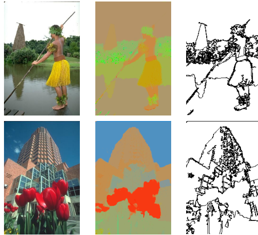
Figure 6.5: Segmentation results obtained with interactive evolutionary optimized of the alpha function parameters.
