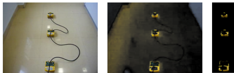
Figure 4.5: Robot detection. Left, original image. Right, the resulting image segmentation. Middle, the result of the SF2 process.
