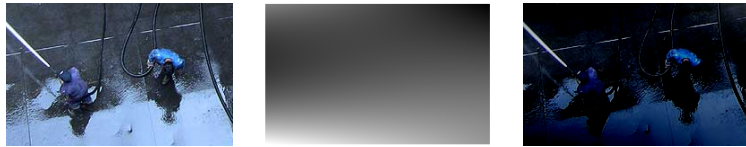
Figure 3.7: Detail from figure 4 images. From left to right: original image, estimated specular bias, corrected image obtained removing the specular field.
