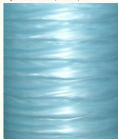
Weakly Turbulent Vortex Flow (Re = 3027)
