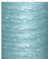
Turbulent Vortex Flow (Re = 8072)
